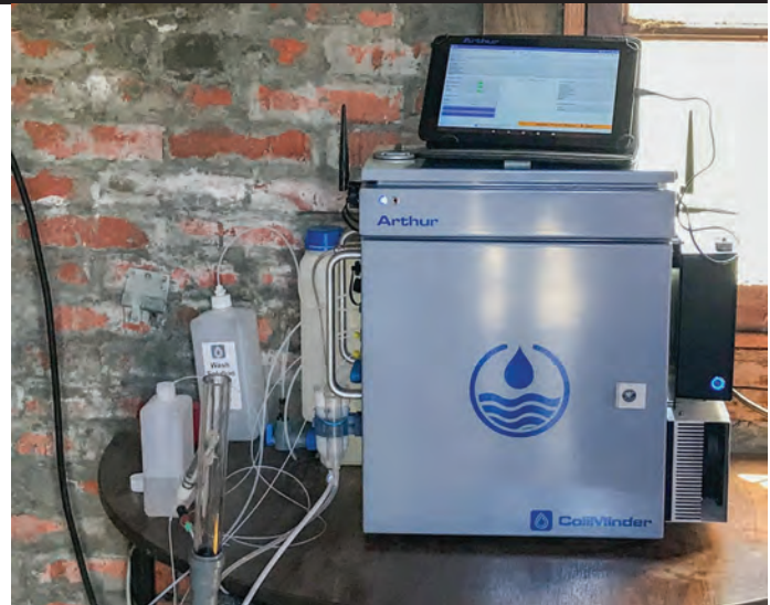
The first ColiMinder installation in Paris monitors E. coli and Enterococci levels in bathing water at Bassin de la Villette
